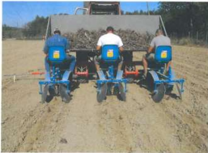
Purpose-built energy cane rhizome planter
