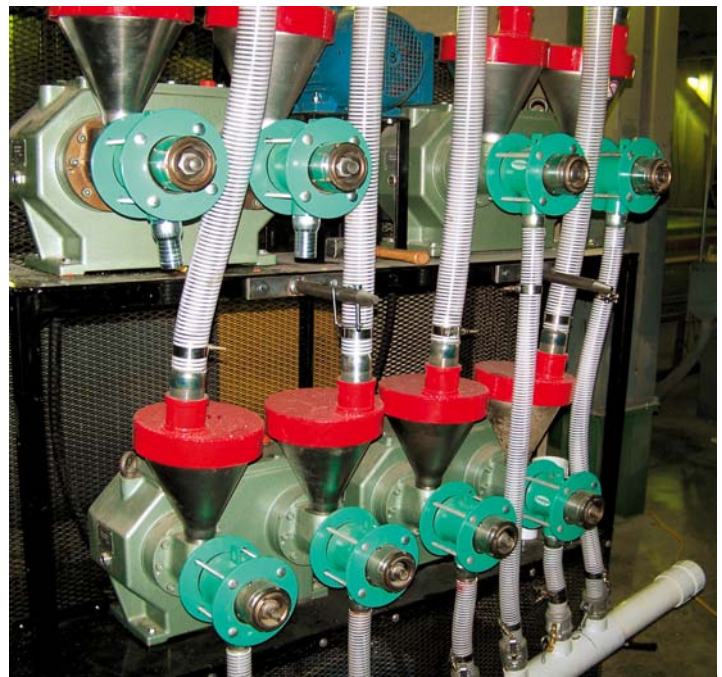
These units crush canola seed at Pendleton Grain Growers Co-op. The resulting oil and meal can be used for biodiesel. USDA Rural Development provided a $300,000 Value-Added Producer Grant for the biodiesel project.
