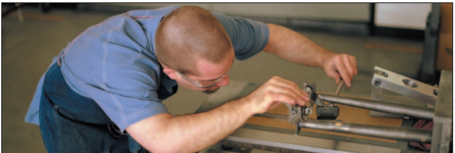
Lots of hand labor, such as proper alignment of bike frames (as seen here in the Burley plant), is required in production of high-quality bicycles.
