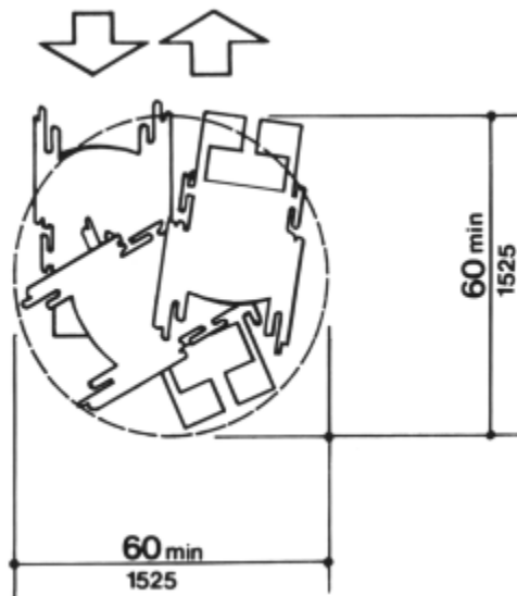
Figure 3(a) Wheelchair Turning Space 60-in (1525 mm) Diameter Space
