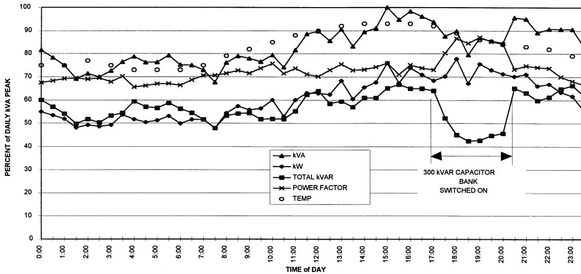
**Figure 7: Effects of 300 kVAR Switched Capacitor Bank**
