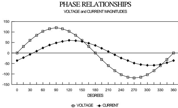
Figure 4: Current Lags the Voltage
