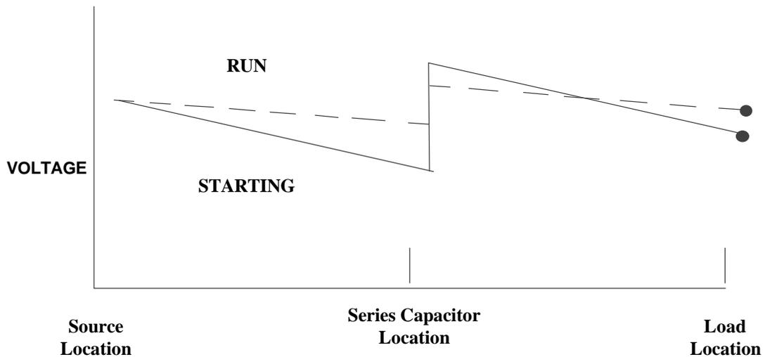
**Figure 17: Motor Starting with Series Capacitor**
