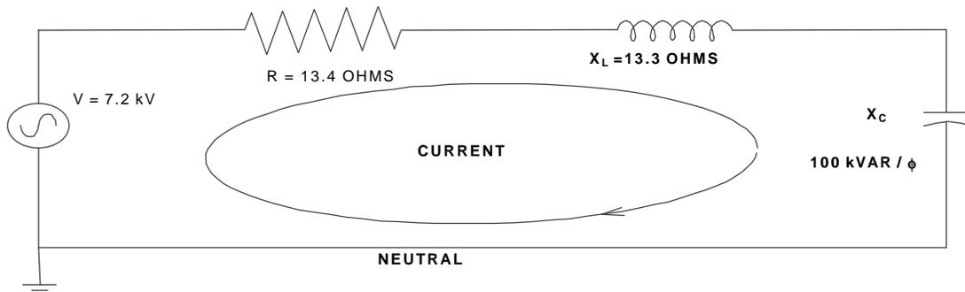
**Figure 12: Voltage Rise from 300 kVAR of Capacitors**
