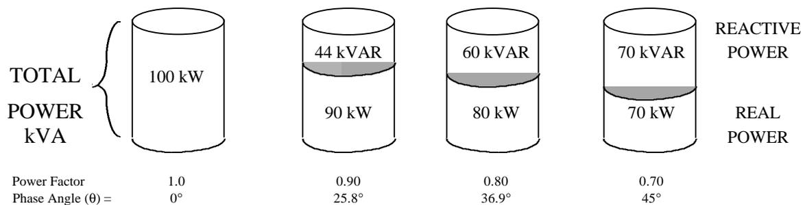
*100 kVA loads at various power factors. kW is usable power. As power factor increases, the useful power delivered is increased. As can be seen, lagging kilovars may form an appreciable component of the system load.*
