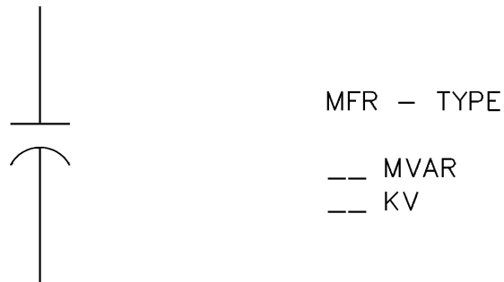
Figure 3-17: Shunt Capacitor. Ref. IEEE Std. 315. Fig. 2.2.11. Copyright © 1975. IEEE. All rights reserved.
