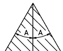
SINGLE MAST OR SHIELD WIRE
