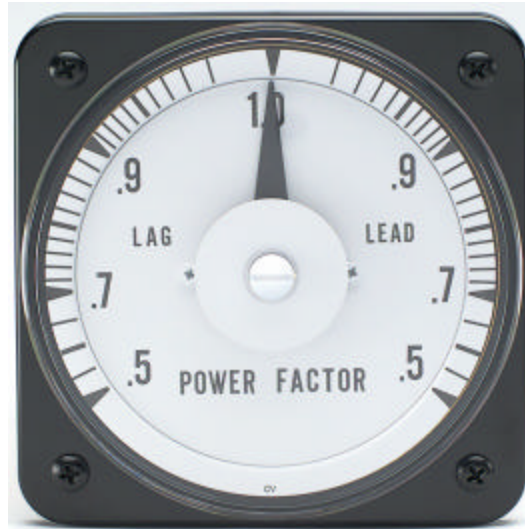
Figure 13-2: Nonlinear Scale Power Factor Meter. Courtesy of Yokogawa.
