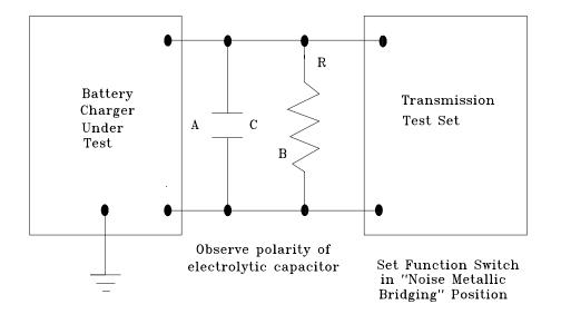
The manufacturer may elect to eliminate the capacitor C from the measurement.
