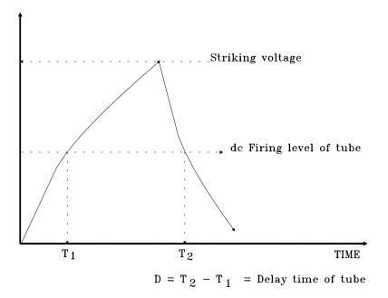
The delay time is that period of time when the potential across an arrester exceeds its dc firing level.
