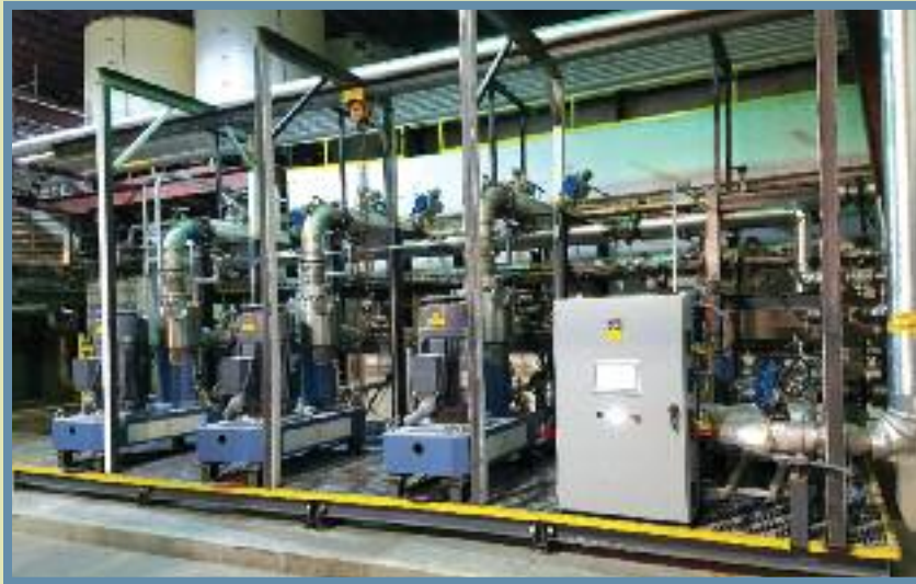
This new machinery at Siouxland Energy Cooperative's (SEC) ethanol plant allows the co-op to process the cellulosic portion of corn kernels into ethanol, resulting in 3 percent more fuel from every bushel of corn. Photo courtesy SEC
