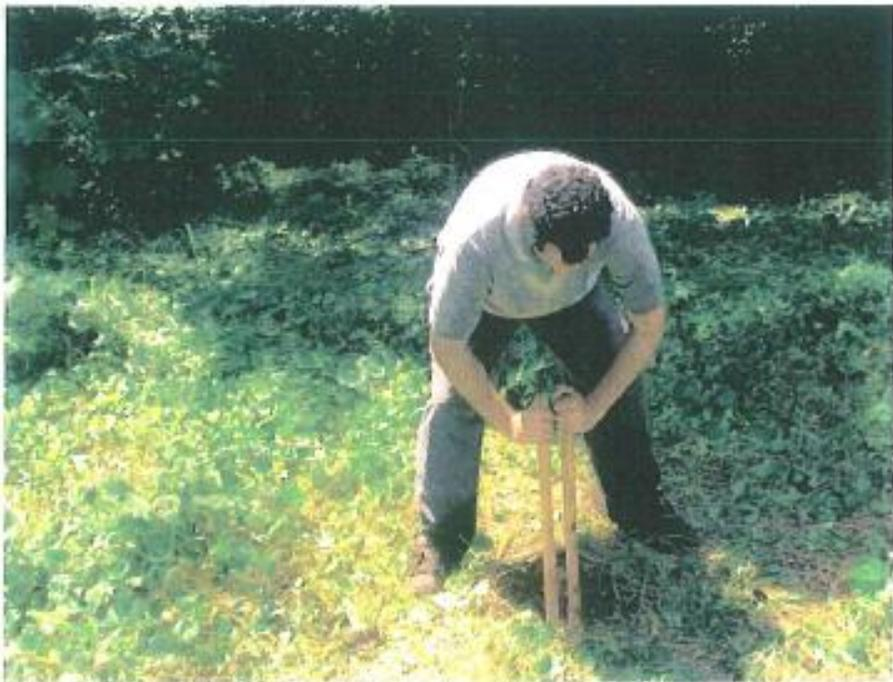
**Photo 7.** Test pit excavation using a post hole digger. Looking west.
