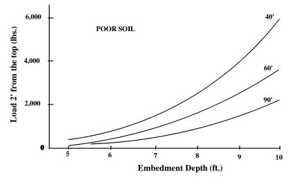
FIGURE 12-1: EMBEDMENT DEPTHS IN POOR SOIL
