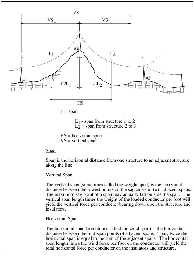
FIGURE 7-4: HORIZONTAL AND VERTICAL SPANS
