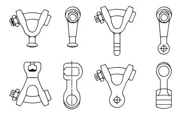
FIGURE 15-7: VARIOUS TYPES OF BALL AND CLEVIS "Y" CONNECTIONS
