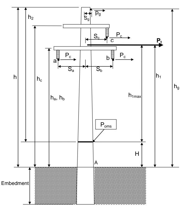
Figure 13-4: TS Type Structure P<sub>OMS</sub>
