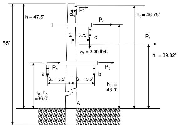
Figure 13-5: TS Type Structure Example
