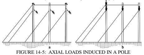
When the structure is considered to be a double deadend or large angle, the poles, guys, and anchors must sustain the full deadend load with an appropriate load factor. For the tangent double deadend shown in Figure 14-6, the poles must sustain the maximum axial load which might occur if all phase conductors on one side of the structure were removed (see Figure 14-6a and 14-6b). However, to "double account" the loads, as shown in Figure 14-6c would be too conservative.
