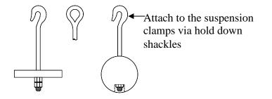
FIGURE 15-13: DISC WEIGHTS (Left), BALL WEIGHTS (Right)
