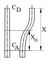
FIGURE 13-13: LOCATION OF POINT OF CONTRAFLEXURE
