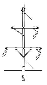
FIGURE 15-18: SMALL ANGLE STRUCTURE WITH SWING ANGLE BRACKETS
