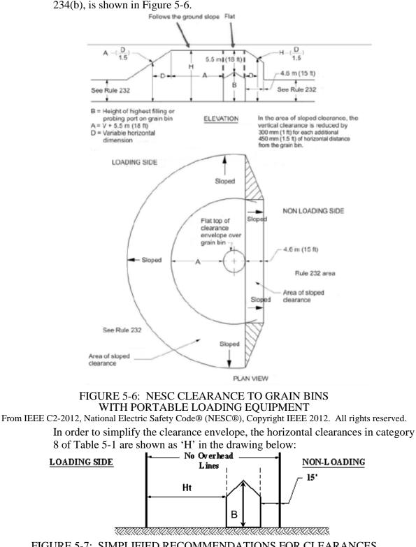
The clearance envelope for portable loading equipment from NESC Figure 234(b), is shown in Figure 5-6.
