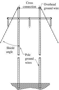
FIGURE 8-4: SHIELDING ANGLE, POLE AND OVERHEAD GROUND WIRES
