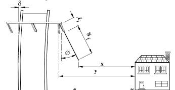
FIGURE 5-1: HORIZONTAL CLEARANCE REQUIREMENT TO BUILDINGS
