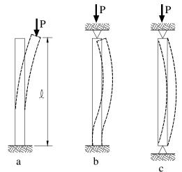
FIGURE 14-3: EFFECTIVE UNBRACED LENGTH FOR VARIOUS END CONDITIONS
