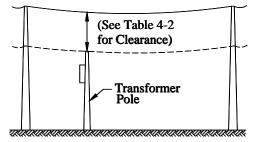
FIGURE 16-3: USE OF A SEPARATE POLE TO MOUNT A DISTRIBUTION TRANSFORMER
