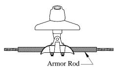
FIGURE 15-9: ARMOR RODS USED WITH SUSPENSION INSULATORS
