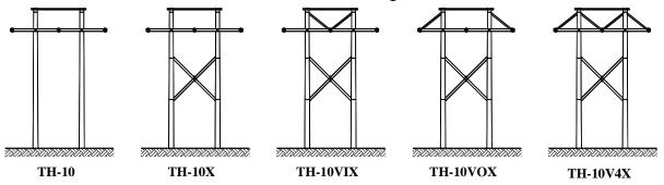
FIGURE 13-15: POLE TOP BRACING ARRANGEMENTS ('X' added to the pole top assembly nomenclature refers to crossbrace)
