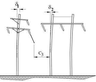
FIGURE 5-11: CLEARANCE BETWEEN CONDUCTORS OF ONE LINE AND STRUCTURE OF ANOTHER
