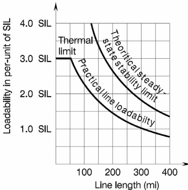
**Note:** The above transmission line loadability curve is for 60 Hz uncompensated overhead lines, and based on Figure 6.1.2 from *Power System Analysis and Design*, Glover/Sarma, at 217 (PWS Publishers 1987). “SIL” refers to “surge impedance load,” which is the power delivered to an electric load that is equal to a transmission line’s characteristic impedance. For a 230 kV line, the SIL is approximately 145 MW.
