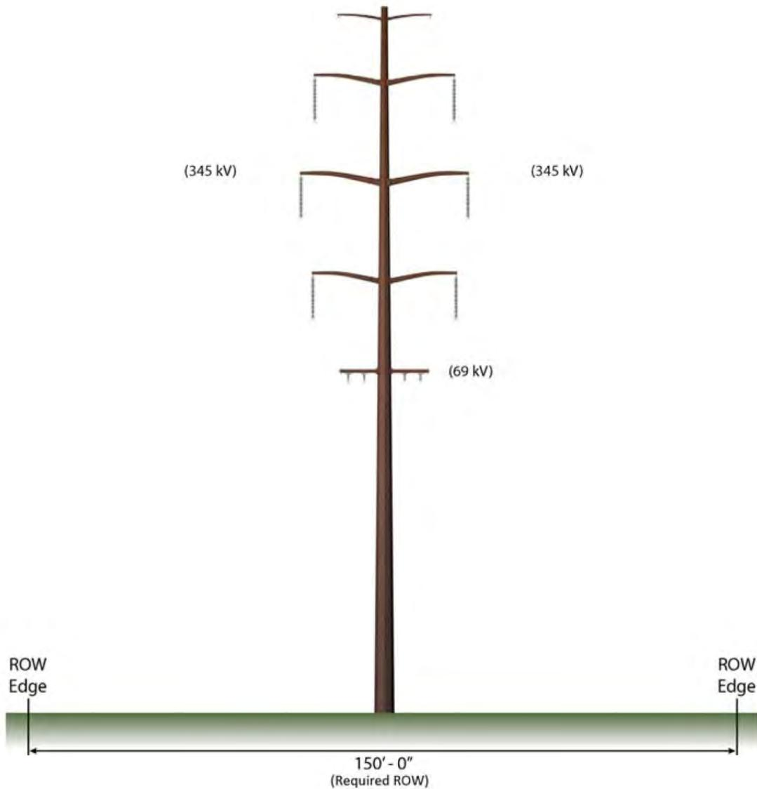
**Figure 2-11: Typical Double-Circuit 345/345 kV Structure with 69 kV Underbuild**
