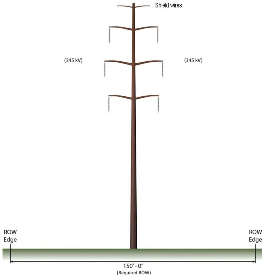
**Figure 2-10: Typical Double-Circuit 345 kV Single-Pole Structure (Davit Arm)**
