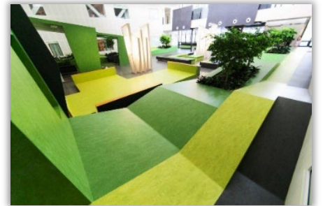
Biobased linoleum made from linseed oil, pine rosins, wood flour
