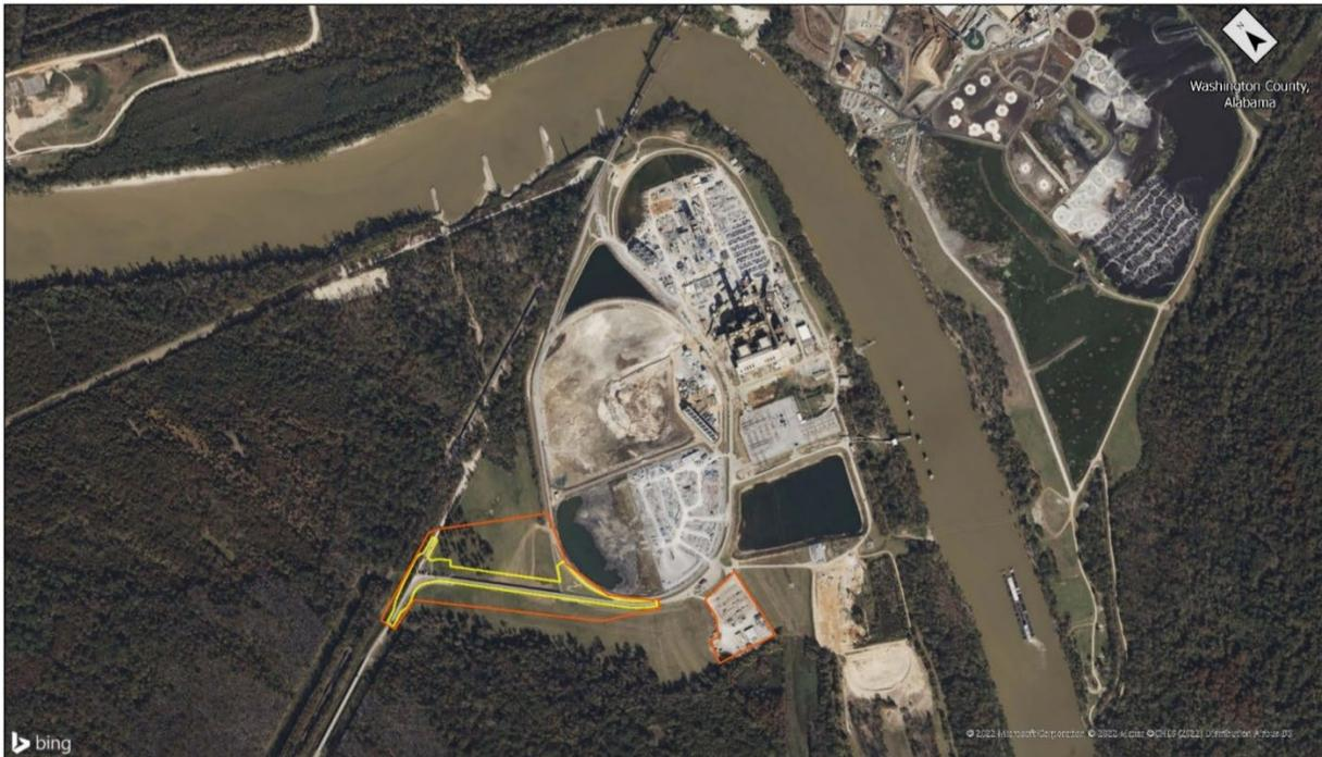
**Figure 1-1 Aerial view of the LEC bridge replacement Project area, showing the proposed bridge corridor (in yellow) and potential environmental impact area (in red), including laydown areas.**
