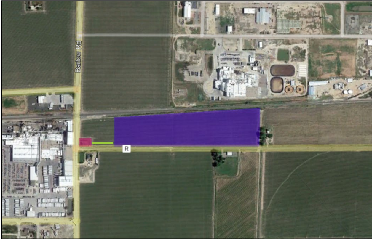
Proposed Project Area in Relation to Municipal Substation/Point of Interconnection (Project area shown in purple and municipal substation shown in pink, buried electric line to point of interconnection shown in green)
