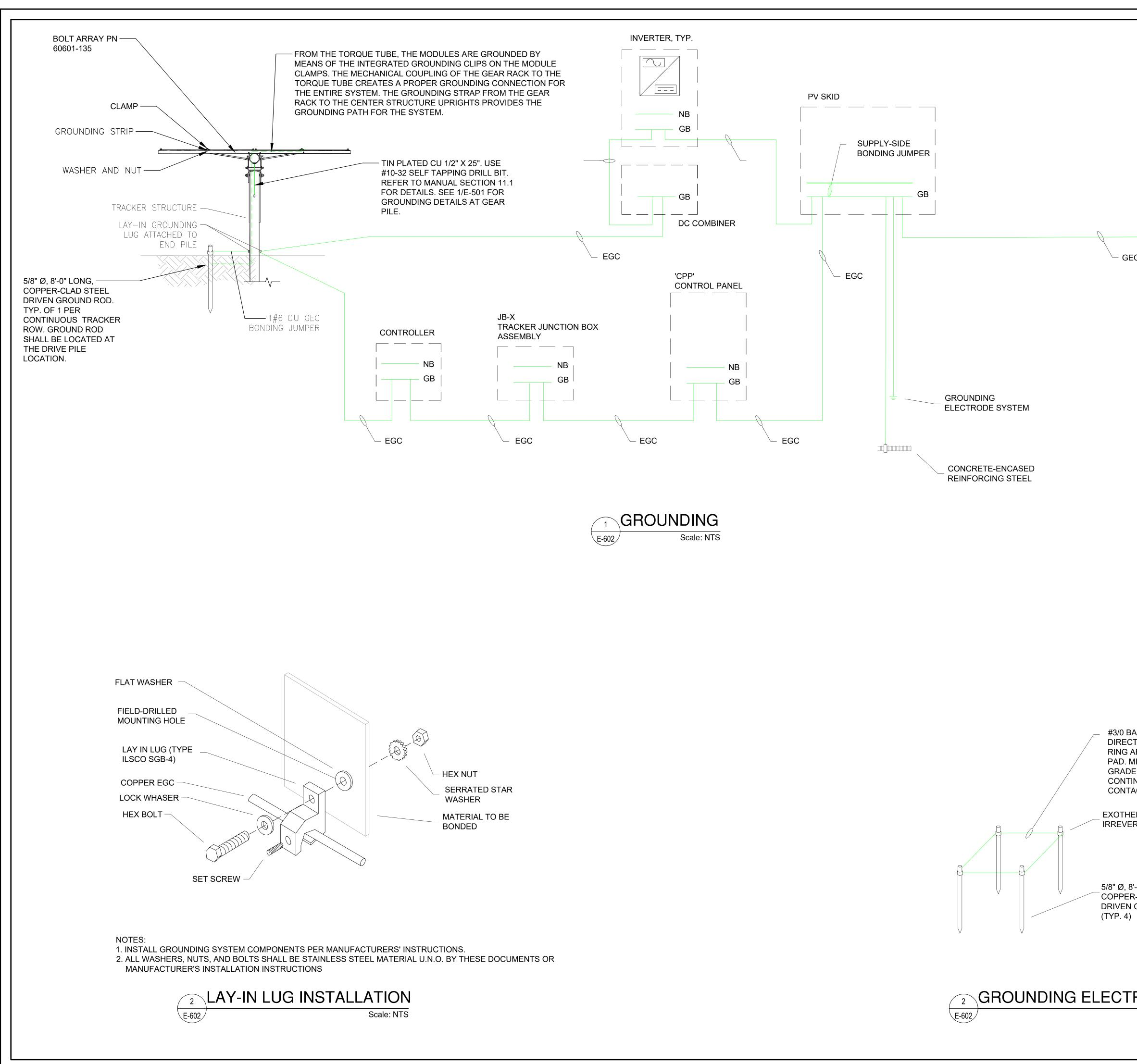
GROUNDING ELECTRODE SYSTEM Scale: NTS
