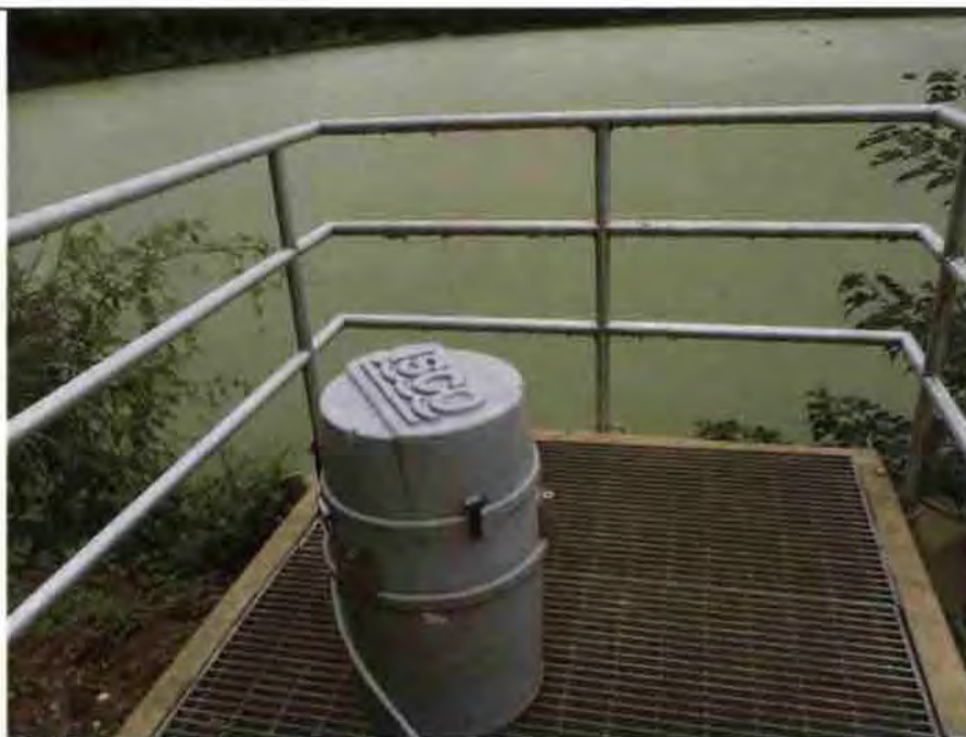
ISCO composite sampler at effluent prior to discharge to facility's sprayfield.
