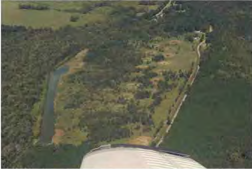
Aerial picture of Uniontown Lagoon Sprayfield #1 - note pooled wastewater (left)
