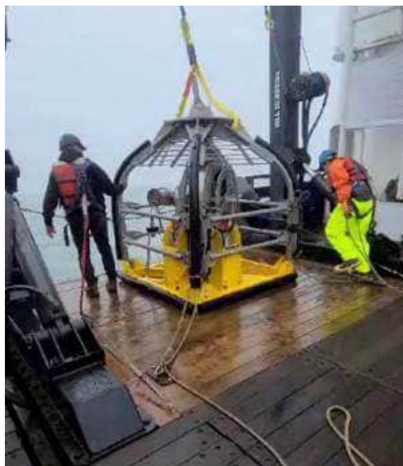
Figure 9-2 Datem Neptune 3000 Cone Penetrometer Test (CPT) system
