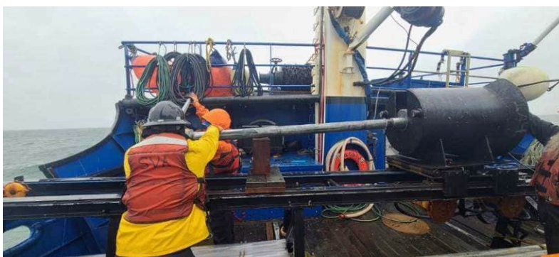
Figure 9-1 Mooring Systems Inc. PC-300 Piston Corer on SVA's custom piston core launch and recovery system
