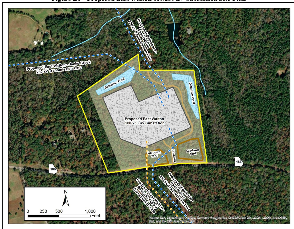
Figure 2.0 – Proposed East Walton 500/230 kV Substation Site Plan
