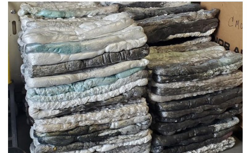
Polystyrene packaging is compressed and flattened into ingots at the NEK WMD transfer station. After processing, they're bagged and sold to a construction company for use as building insulation.
