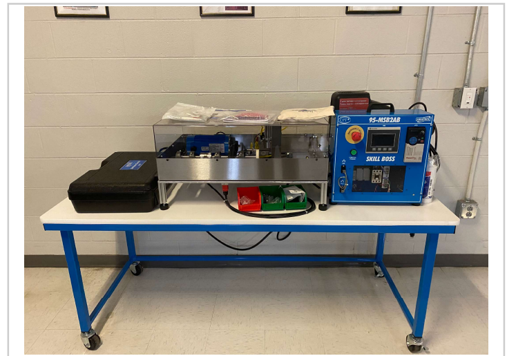
The Amatrol Skill Boss is used by the Manufacturing Skill Standards Council for its Certified Production Technician (CPT) Plus certification in electronic, electrical, fluid power, and mechanical systems.
