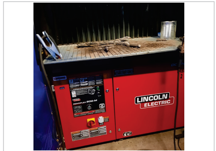
One of the Lincoln Electric Downflex 200-M Weld Fume Downdraft Tables purchased for the welding program at Clarkrange High School.
