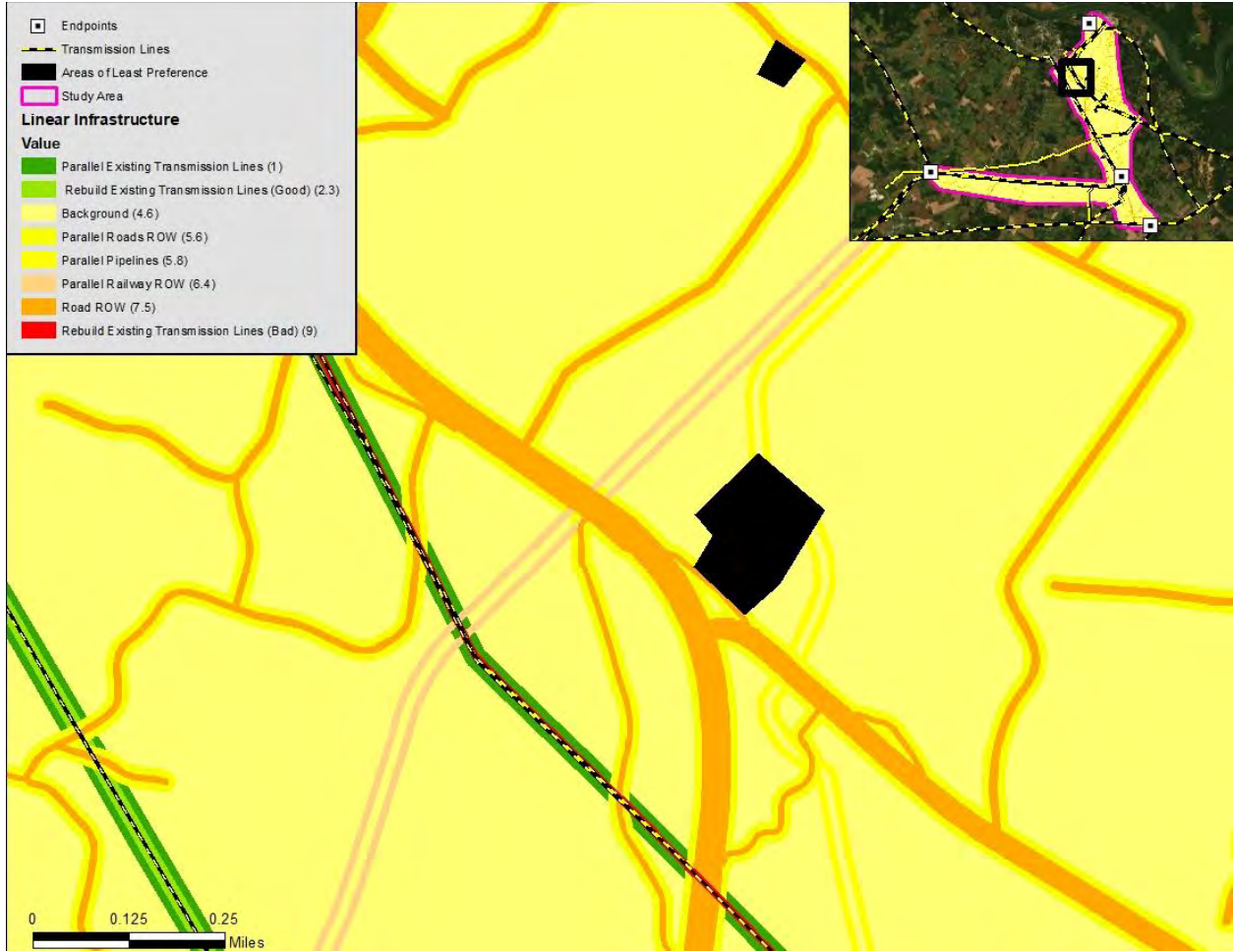
Figure 20 Linear Infrastructure Suitability Grid
