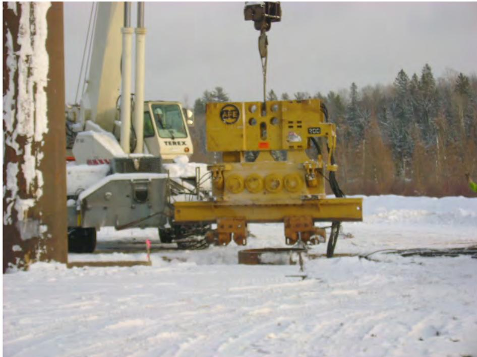
**Ground Based Vibratory Caisson and Hammer Unit**
