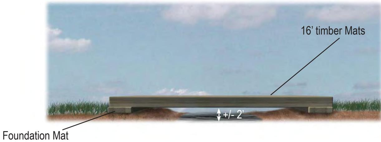
Figure 3: Representative Drawing of Temporary Clear Span Bridge
